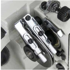
打线凸轮外置 External cable & cam
