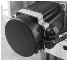
步进电机控制针距 The stepping motor controls the stitch length
