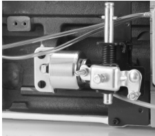
全新膝靠抬压脚结构 New knee lift presser foot structure
