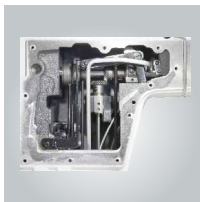
全新膝靠抬压脚结构 New knee lift presser foot structure
