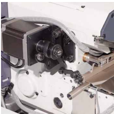
步进驱动，剪线，抬压脚声音轻 Stepper adjustment of stitch length, presser foot lifting, thread trimming,
