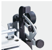
上差动调节 top differential adjusting.
