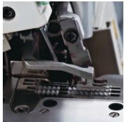
上差动送料牙 top differential feed dog.
