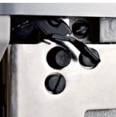
外置针距按钮 External stitch length button
