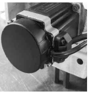
步进电机控制针距 The stepping motor controls the stitch length
