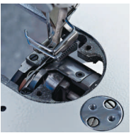
圆刀剪线 Round thread trimmer
